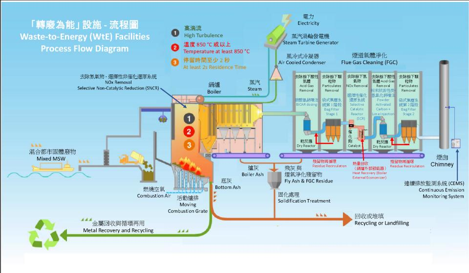
Development of Integrated Waste Management Facilities Phase 2 – Process Flow Diagram of Waste-to-Energy Facilities
