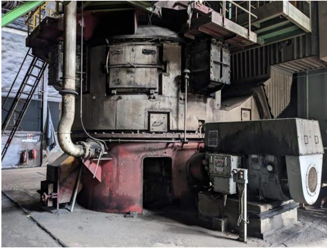
Photo 7: A coal grinding mill at unit A4
