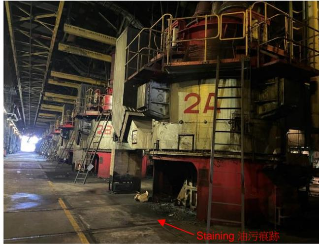
Photo 8: A series of coal grinding mills along CPA Station Building
