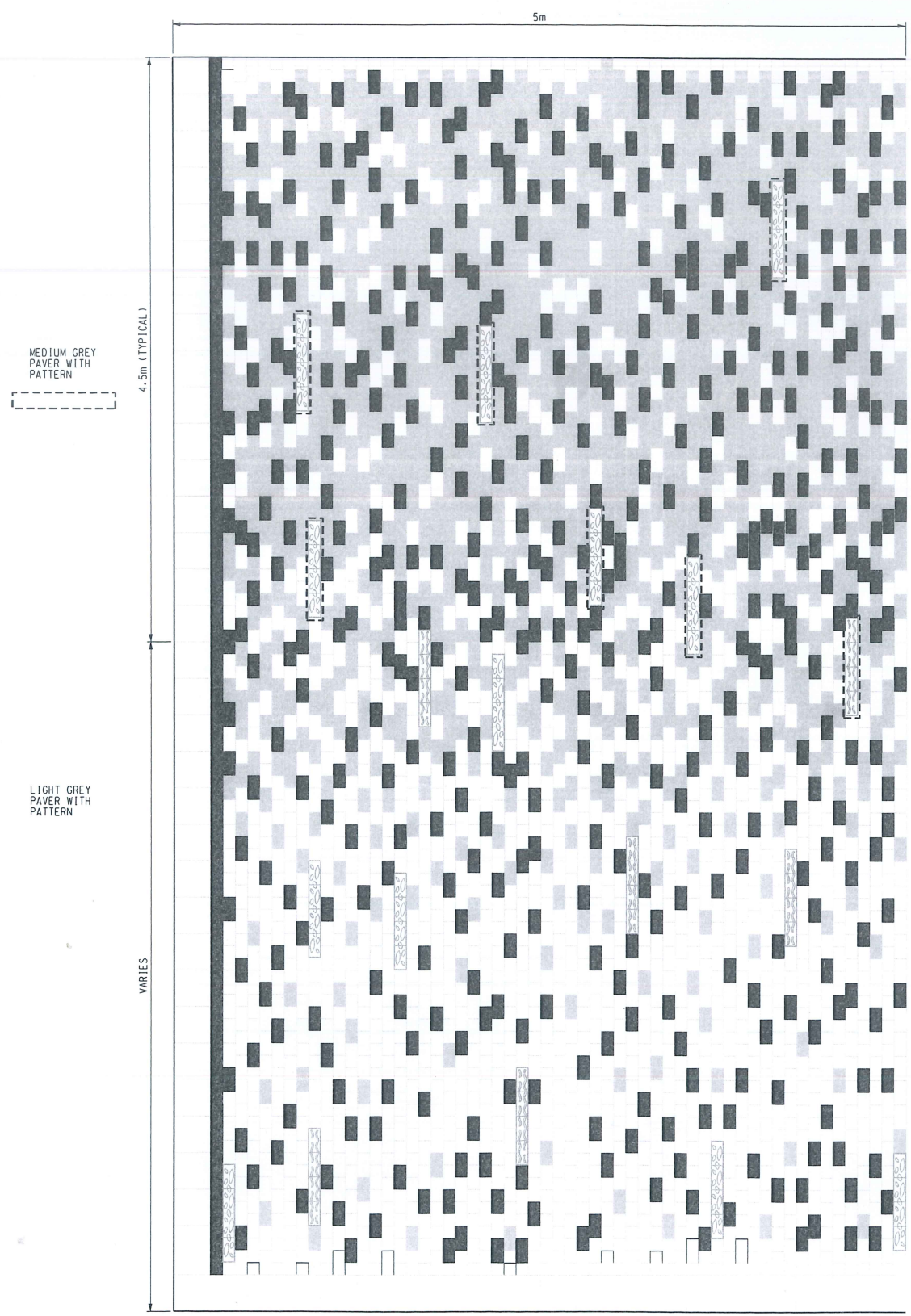
TYPICAL PAVING PATTERN MODULE
