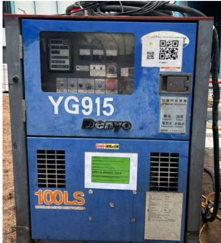
Photo 2: Power Mechanical Equipment with Quality Power Mechanical Equipment (QPME) labels were used at site to lower the noise nuisance to the nearby residents.
