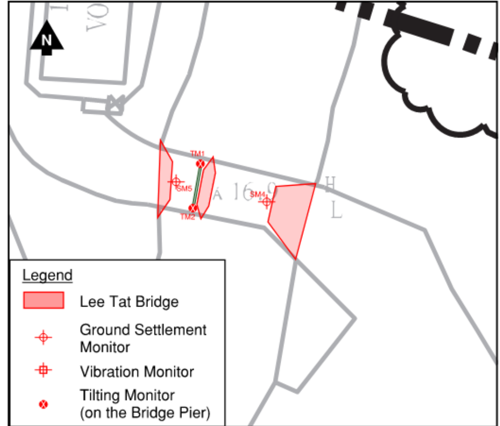
Monitoring Point (Below Bridge Deck)
