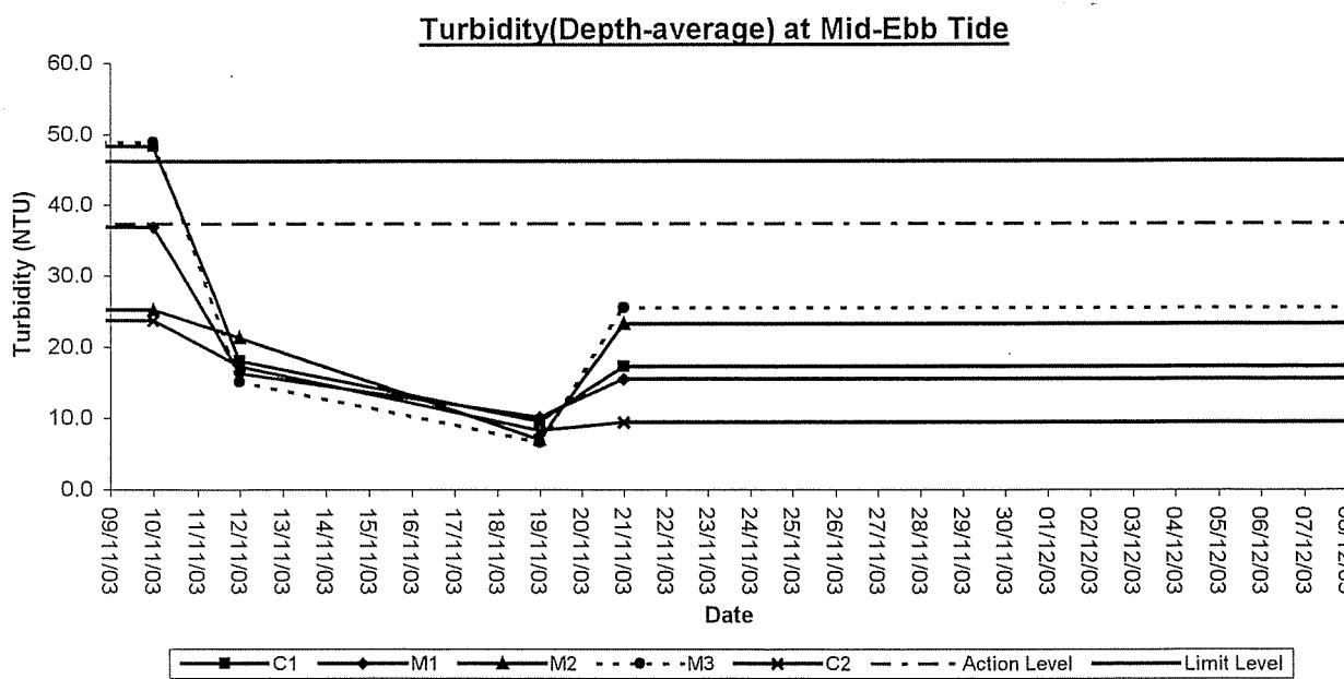
Remark: No exceedance of Action Level was found at 10/11/03 since the Turbidity at C1 was less than 120% of Upstream Control Location M3.
