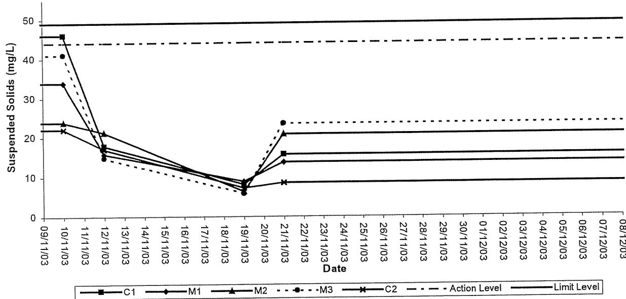
Remark: No exceedance of Action Level was found at 10/11/03 since Suspended Solids at C1 was less than 120% of Upstream Control Location M3.
