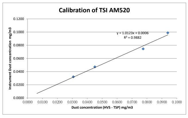
\*\*\* Filter paper being used in the calibration : 209603, 209604, 209605, 209606 Those filter papers are weighted by HOKLAS laboratory (ALS Technichem (HK) Pty Ltd.)
