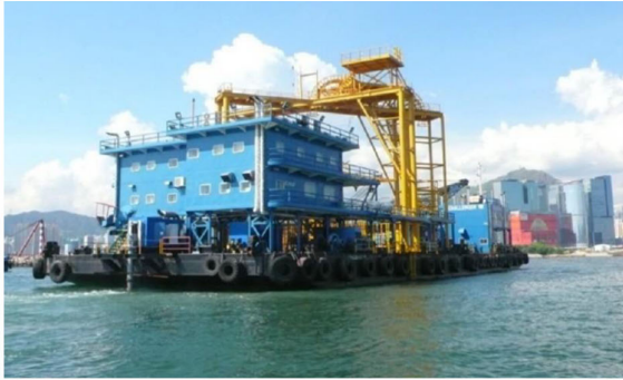
Typical Cable Installation Barge / Vessel using Injector Burial Tool
