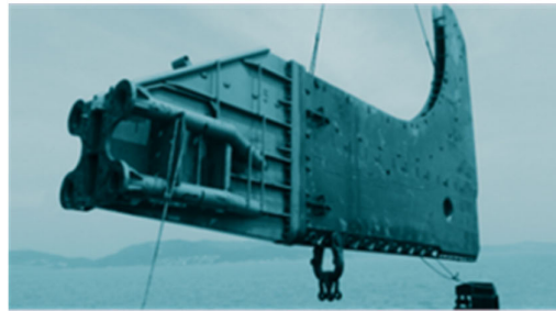
Typical Injector Burial Tool
