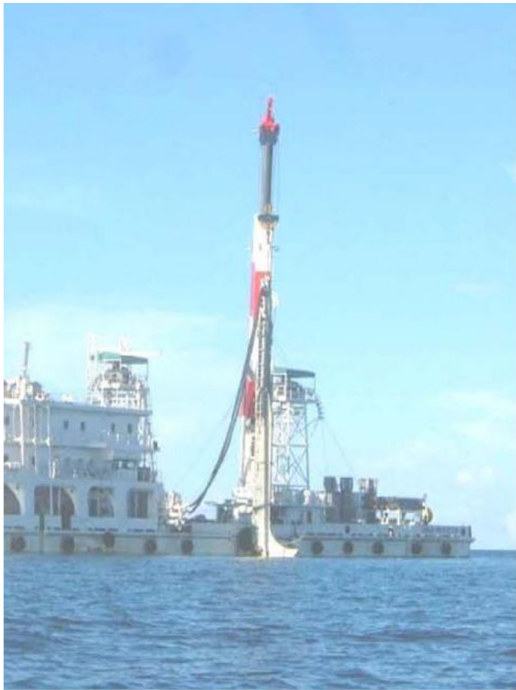
Typical Injector Burial Tool
