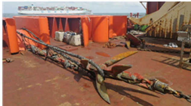
Typical Grapnel (e.g. for Route Clearance)
