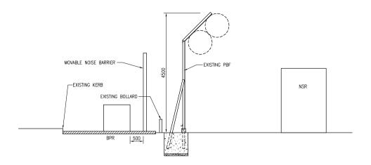
TYPICAL SECTION OF MOVABLE NOISE BARRIER DURING EXCAVATION, FOOTING CONSTRUCTION AND ROAD CONSTRUCTION
