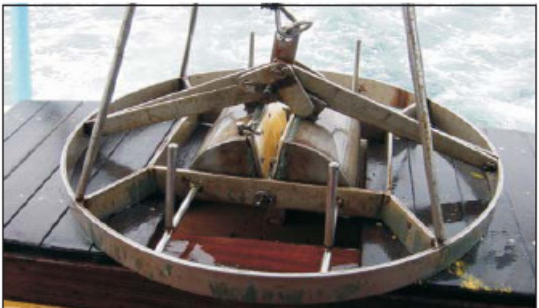
Modified Van Veen grab as used to collect samples at Black Point and the Study Area
