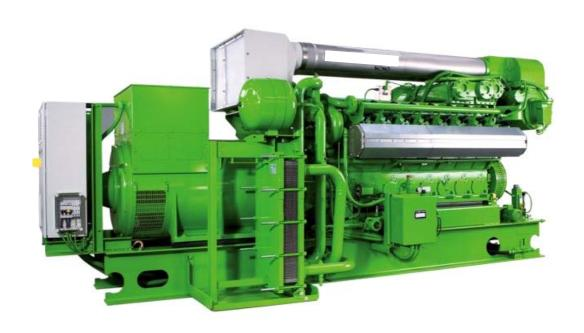
Electrical output 851 kW el. Thermal output 982 kW
